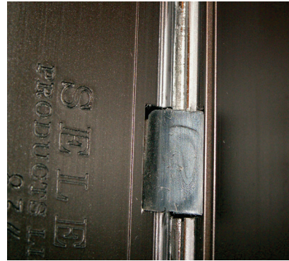
SELECT hinge bearing shows minimal wear after 25,000,000 cycles (only 30 one-thousandths of an inch drop).
