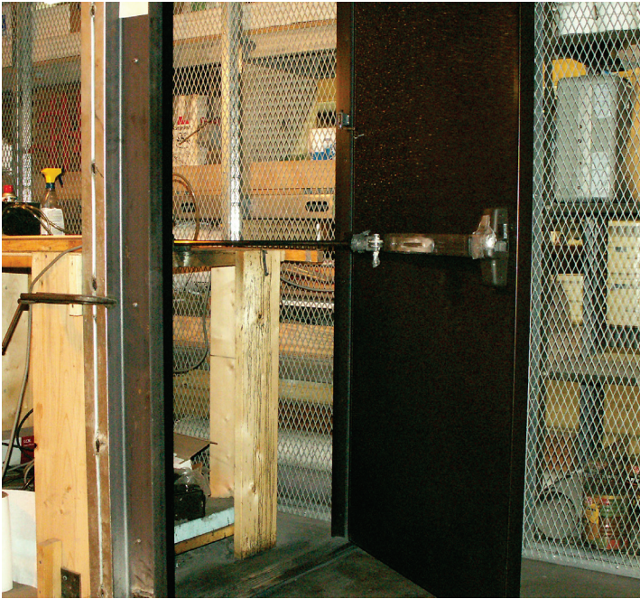
Front view of FRP door and channel iron framework assembled for cycle testing.
