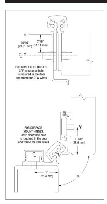
**PREP:** SELECT geared continuous hinges can be prepared for concealed electric through-wires to provide continuous current. Through-wires available in sets of 4, 5, 8, 10 or 12.
