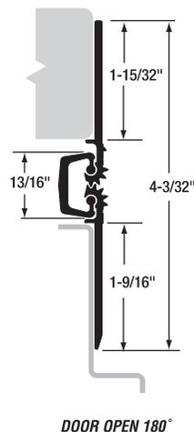
**MATERIAL:** Extruded 6063 T6 aluminum alloy with self-lubricating polyester thrust bearings.
