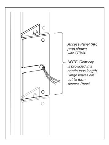
**PREP:** SELECT geared continuous hinges can be prepared with hinge leaf panels to allow easy access to electrical components while preserving gear cap's appearance.
