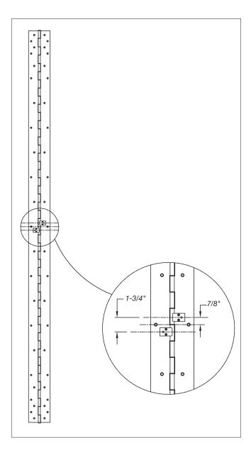
PREP: SELECT pin & barrel continuous hinges can be prepared for concealed electric through-wires to provide continuous current. 28 gauge through-wires with ElectroLYNX™ connectors available in sets of 4 (EL-4), 8 (EL-8) or 12 (EL-12).
