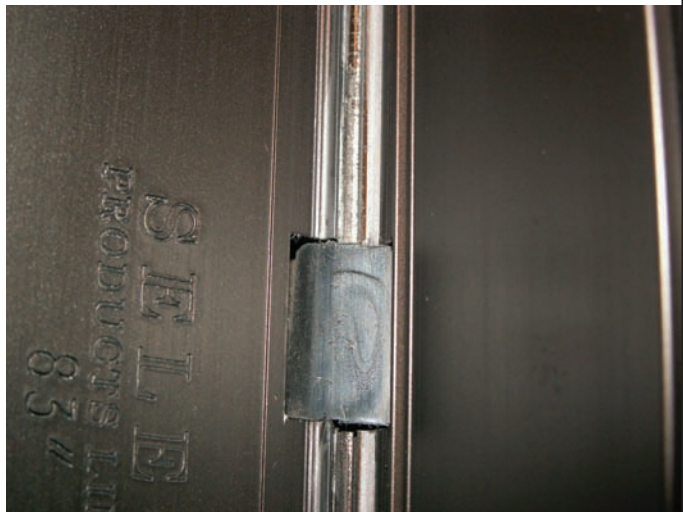
Above: The last of three cycle counters installed on an FRP door equipped with SELECT's SL11 geared continuous hinge. Two counters were replaced before reaching 25,000,000 cycles.
