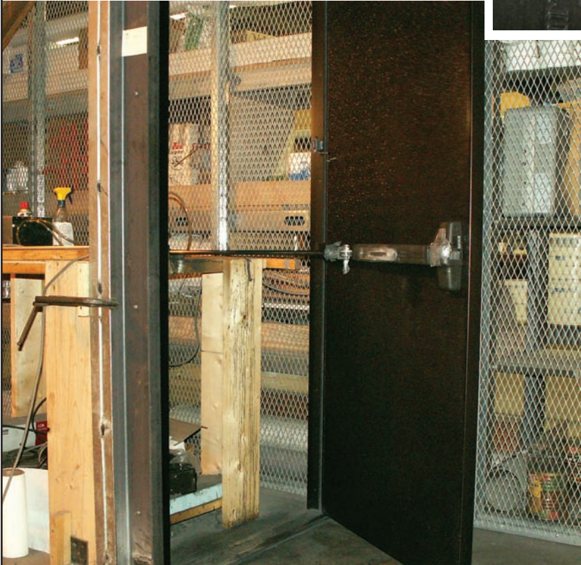
Below: Front view of cycle test setup in operation at Architectural Testing, Inc., St. Paul, MN.
