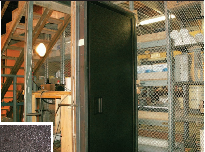
Above: Front view of FRP door and channel iron framework assembled for cycle testing.
