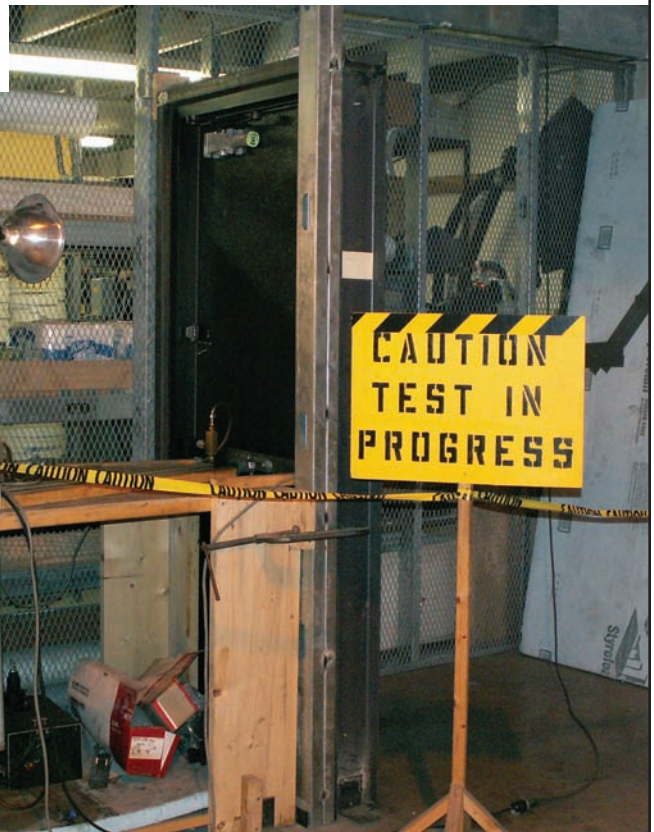
Below: Cycle test setup at Architectural Testing, Inc., St. Paul, MN. Note the empty packaging from two door closers. The first of two failed door closers was replaced after only 4,803,830 cycles.
