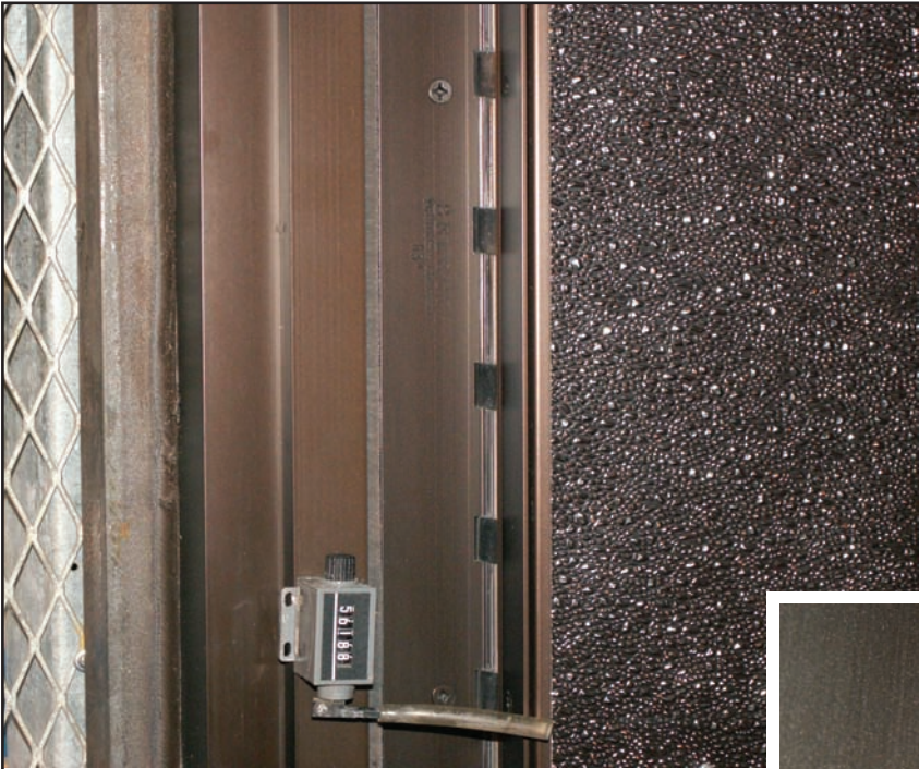
Above: The last of three cycle counters installed on an FRP door equipped with SELECT's SL11 geared continuous hinge. Two counters were replaced before reaching 25,000,000 cycles.
