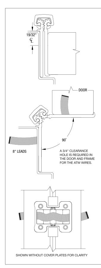
**PREP:** SELECT geared continuous hinges can be prepared for accessible electric through-wires to provide continuous current. Through-wires available in sets of 4, 8 or 12.
