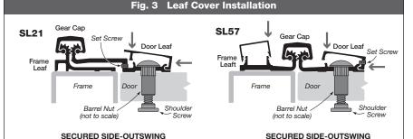
**NOTE:** For inswing applications, reverse position of barrel nut and shoulder screw so that the shoulder screw is on the secured side of the door.
