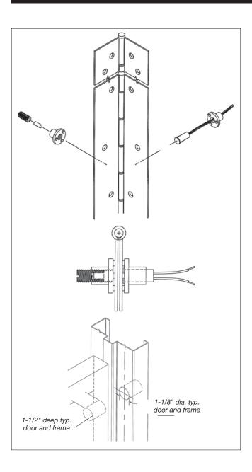
**PREP:** SELECT pin & barrel continuous hinges can be prepared for the adjustable concealed monitor switch. Rigid welded assembly gives you the ability to adjust the AMS to work with all applications.
