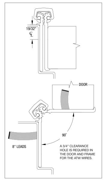
**PREP:** 4-1/4 inch panel as a retrofit option to electrify an existing concealed hinge or fix a failed electronic entryway. Through-wires available in sets of 4, 8 or 12.
