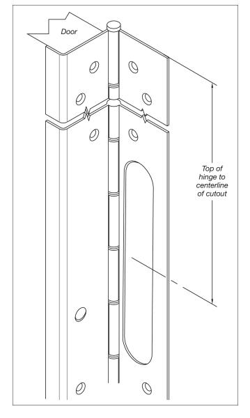
**PREP:** SELECT pin & barrel continuous hinges can be prepared for Adams Rite 4612 power transfer unit.
