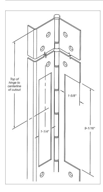
**PREP:** SELECT pin & barrel continuous hinges can be prepared for Von Duprin power transfer unit.
