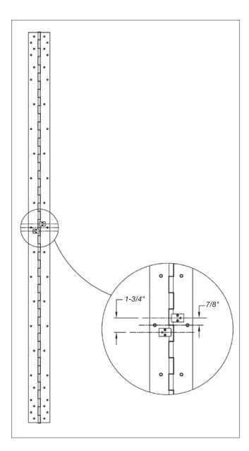
PREP: SELECT pin & barrel continuous hinges can be prepared for concealed electric through-wires to provide continuous current. 28 gauge through-wires with ElectroLYNX<sup>™</sup> connectors available in sets of 4 (EL-4), 8 (EL-8) or 12 (EL-12).
