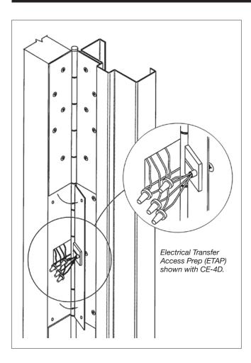
**PREP:** SELECT pin & barrel continuous hinges can be prepared with hinge leaf panels to allow access to electrical components.
