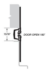
**MATERIAL:** Extruded 6063 T6 aluminum alloy with self-lubricating polyester thrust bearings.
