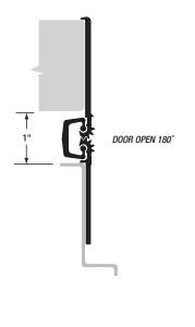
**MATERIAL:** Extruded 6063 T6 aluminum alloy with self-lubricating polyester thrust bearings.
