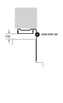
**MATERIAL:** 14 gauge 304 stainless steel barrel with 3/16" diameter 304 stainless pin. Long-life nylon medical bearings.
